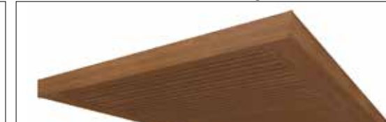
Wood-laminate roof frame + ceiling
